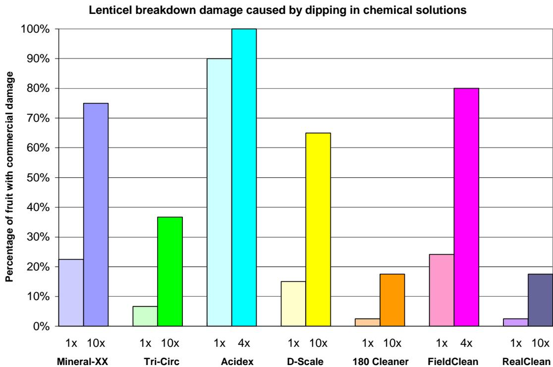
**Figure 3.** Effect of packingline chemicals and concentration on commercially unacceptable LB damage—fruit dipped in solution and not rinsed (Experiment I—Laboratory Study).
