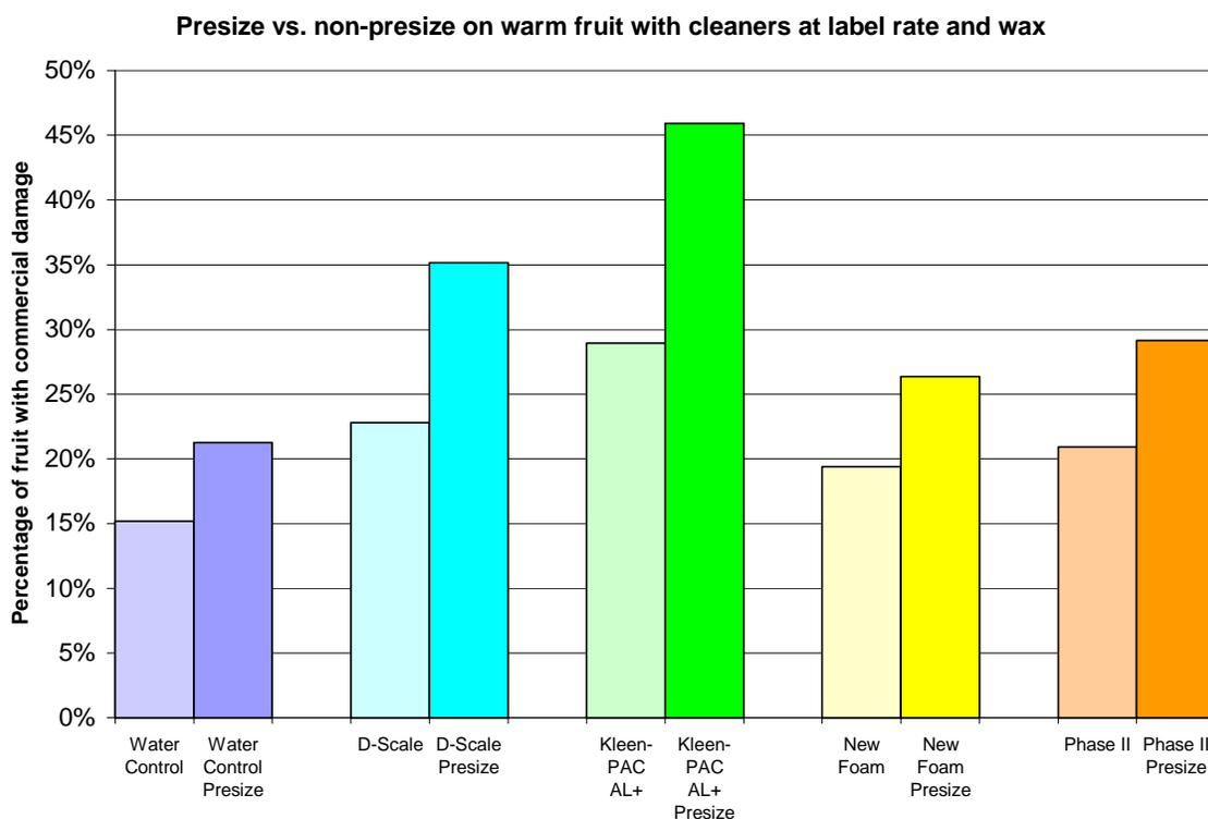
**Figure 6.** Effect of cleaner and presize on commercially unacceptable LB damage—warm fruit with a warm rinse and waxed with carnauba or shellac (Experiment III—Packingline Study II).
