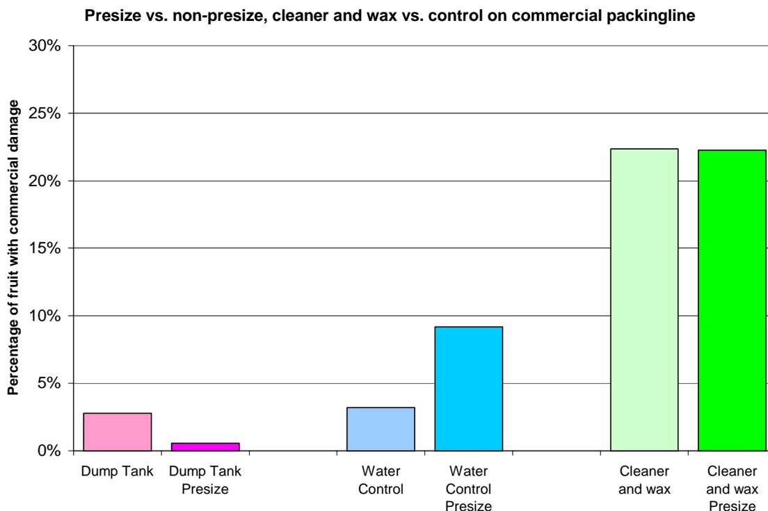
**Figure 8.** Effect of presize, cleaner and wax on commercially unacceptable LB damage—commercial packingline (Experiment IV—Commercial Packingline Study).
